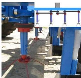
Figure 32 Powered residue-throwing finger no-till seeder
