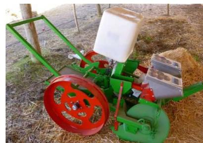
Figure 6 Angled single disc seed drill
