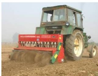
Figure 23 Strip rotary hoe mini-till seeder
