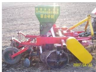
Figure 30 Powered straight knife mini-till seeder
