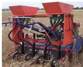
Figure 15 ACIAR modified 2BG-6A rotary tillage seed drill
