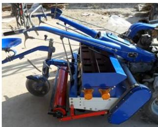
Figure 14 2BFG-100 seed and fertilizer machine
