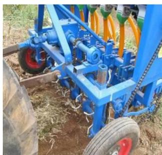
Figure 31 Powered chain no-till seeder
