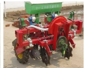
Figure 28 Powered disc mini-till seeder
